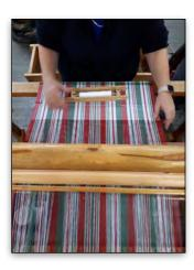
testing the tension of the piece being made to ensure that the thread was neither too loose or too tight and how to use the handle to fit the thread together after each pass.
